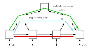
Fig. 5. Architecture of sub-logarithmic adder.
