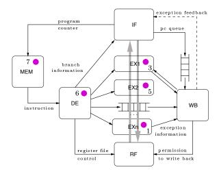
Fig. 2. The MiniMIPS pipeline structure.
