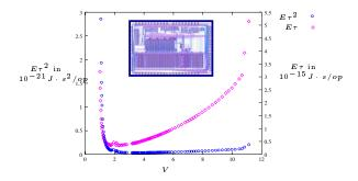
Fig. 1. Measured joint energy/cycle time metrics for the first asynchronous microprocessor over a range of voltages.
