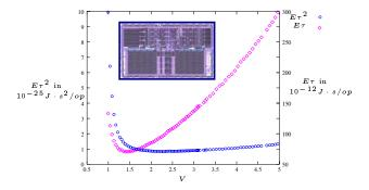
Fig. 4. Measured joint energy/cycle time metrics for the MiniMIPS asynchronous microprocessor over a range of voltages.
