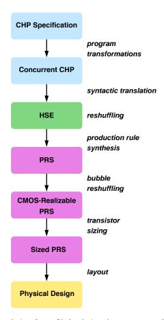
Fig. 6. Top-down design flow. If the design does not meet the required performance/energy/area target, design steps may have to be iterated.
