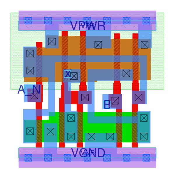
Example from Skywater 130 library for synchronous logic https://antmicro-skywater-pdk-docs.readthedocs.io
