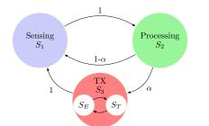
Fig. 1: Semi-Markov Chain for WSN Mote
