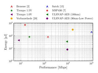
Fig. 7: AES Hardware Energy-Throughput Space
