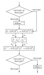
Fig. 5: Composite Field Transformation Byte Substitution
